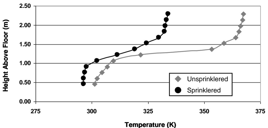
Figure 4: Temperature measurements inside the compartment away from the spraying sprinkler showing two distinct stratified layers in both the unsprinklered and sprinklered cases.
