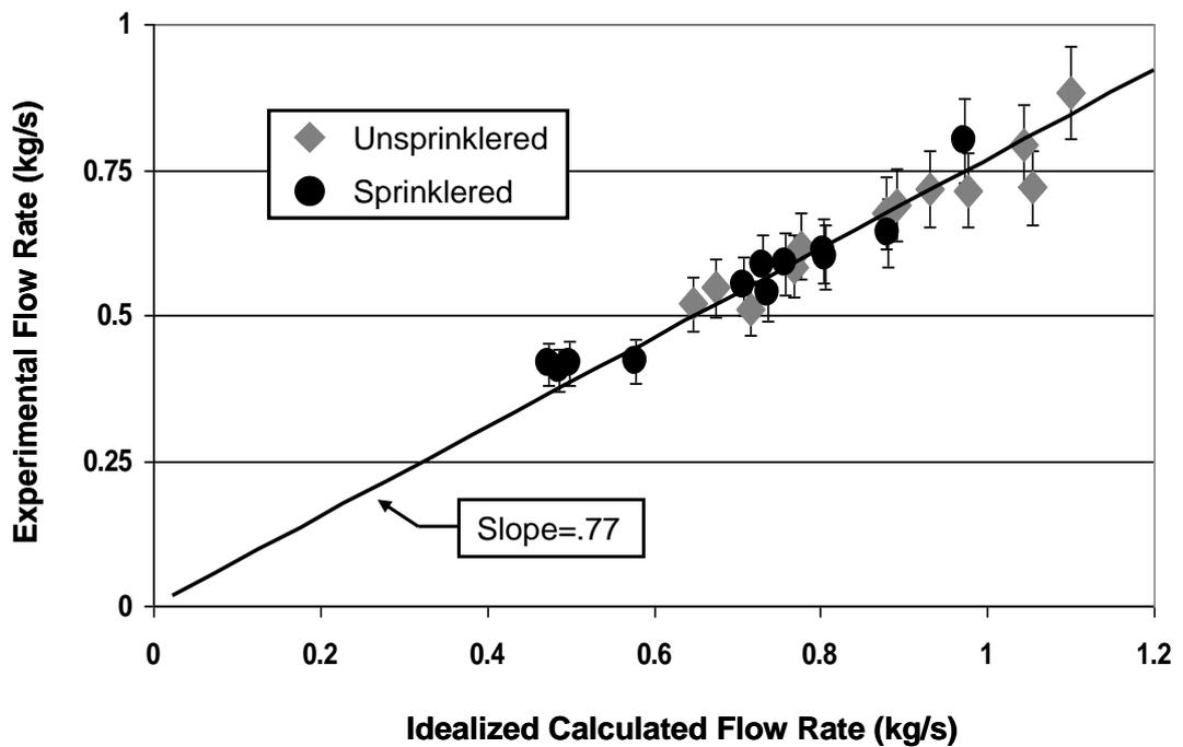
Figure 6: Determination of discharge coefficient with both unsprinklered and sprinklered tests. The  $C_D$  of 0.77 for both cases is very similar to the  $C_D$  of 0.76 for only the unsprinklered case.
